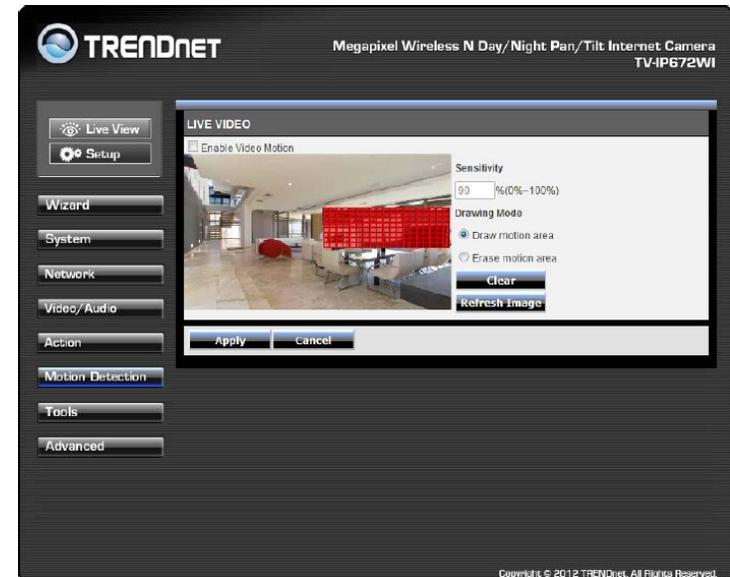
Click the **Enable Video Motion** checkbox to activate motion detection. There are two main fields: **Sensitivity** and **Drawing Mode**. **Sensitivity** is based on the strength of the motion in the designated area. **0%** means the strength is low and the system moves up incrementally to **100%** full sensitive strength.
