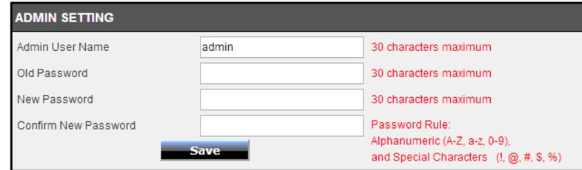
In this section we can configure the **administrator** account's login credentials that will be used to login to the camera's Web UI. In the **Admin User Name** field, enter the login username that will be used for this camera. In the **Old Password** field enter the old/current login password of the camera. In the **New Password** and **Confirm New Password** fields, enter the new login password that will be used for this camera. Click the **Save** button to save the modifications made.
