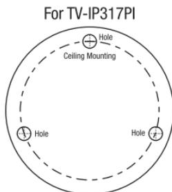
3. Drill holes at each marked position on the template. Make sure the drill bit matches the size of the holes on the template.
