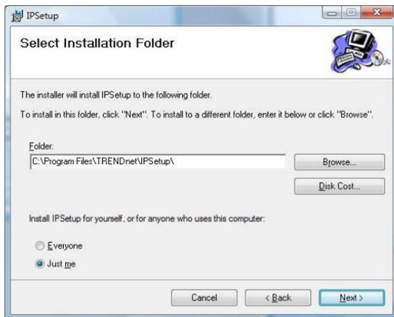
4. Click “**Next**” to confirm the IPSetup software to be installed to the computer.
