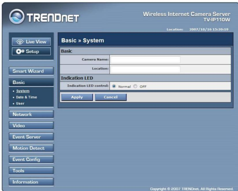
The Web Configuration contains the settings that are required for the camera in the left menu bar, including **Smart Wizard**, **Basic**, **Network**, **Video**, **Event Server**, **Motion detect**, **Event Config**, **Tools**, and **Information**.
