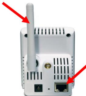
Attach the external power supply to the DC power input connector located on Camera's real Panel, and then connect it to your local power supply.
