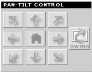
When you connect a pan/tilt camera, the system will detect the camera's function automatically and the PAN-TILT CONTROL buttons will become functional. Otherwise, these buttons are displayed as gray out buttons.
