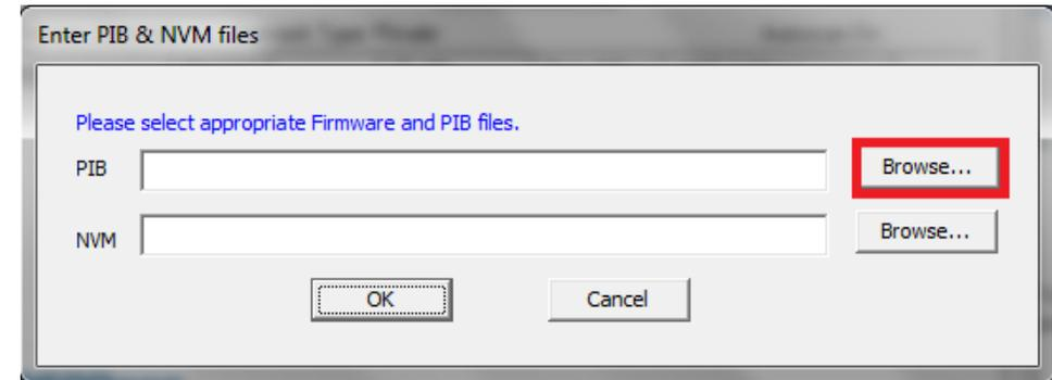
7. Click **Browse** next to the **NVM** field and navigate to the unzipped folder with the firmware files. Select the NVM file. (Ex. TPL-401E-NVM-v5.0.1-0-0-X-FINAL.nvm)
