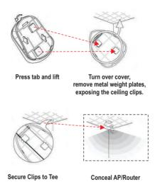
⚠ Note: If the ceiling tees are made of steel, turning the antenna base cover over may not be necessary, because the base has embedded magnets which can be used to adhere the antenna to the ceiling tee.
