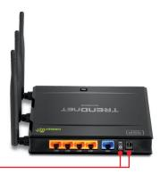
Connect the Power Adapter to the TEW-692GR and then to a power outlet. Move the power switch to the "On" position (EU version only).
