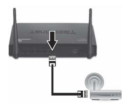
5. Connect one end of a network cable to one of your router LAN ports (1-4). Connect the other end of the network cable to the computer Ethernet port (also called network port).
