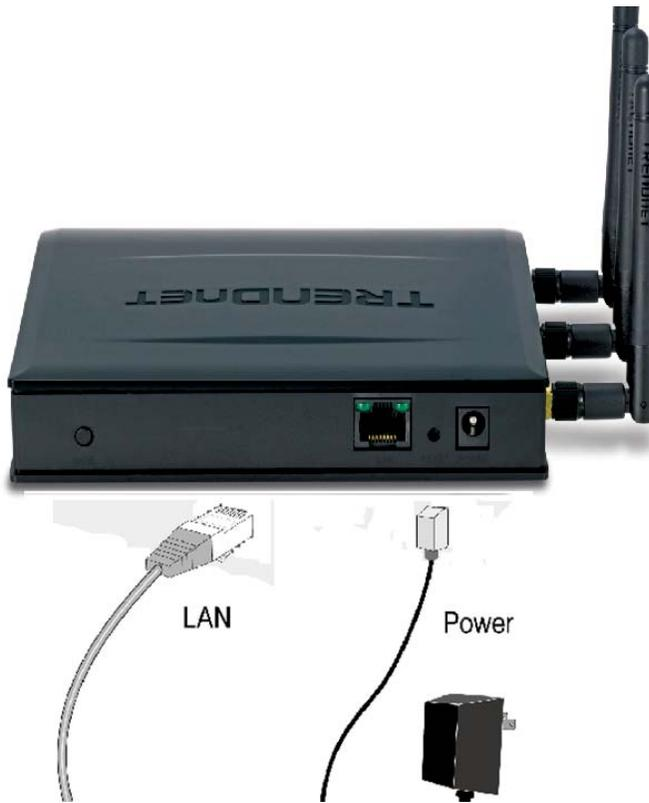
**Figure 4: Installation Diagram**
