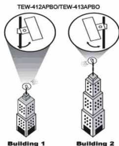
Figure 3.1: Adjusting TEW-412APBO/TEW-413APBO for best reception
