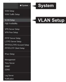
By default, VLAN #1 refers to the LAN interface and the default IP address settings of the router.
