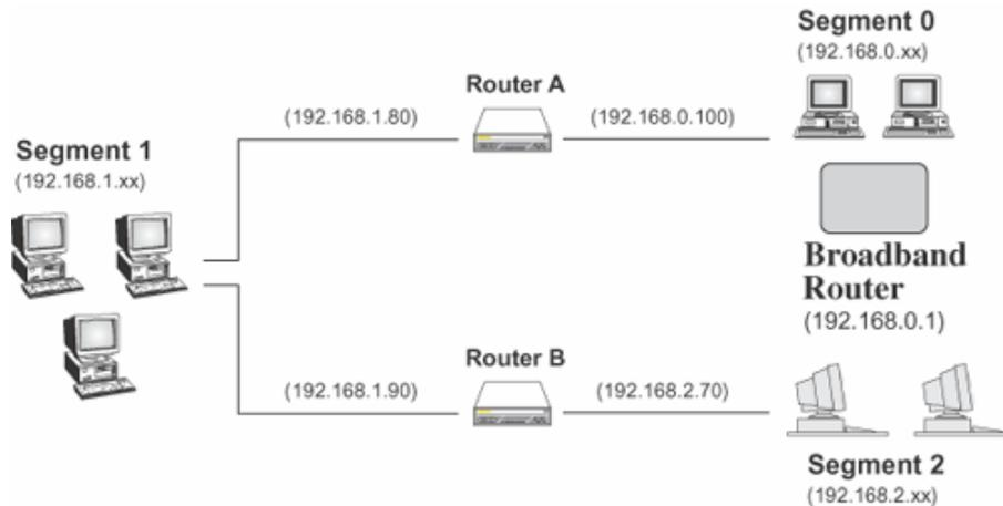
Figure 52: Routing Example
