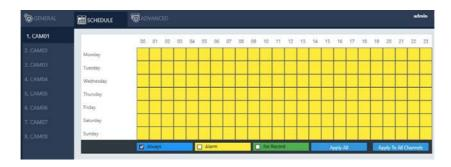
To modify the recording schedule, switch the recording type from **Always** (continuous recording), **Alarm** (record only when an alarm is triggered), or **No Record** (disable recording), and highlight the desired date and time accordingly. Click **Apply All** to apply your selection of recording type to all dates and time.
