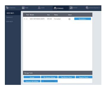
In **HDD MGT**, there are HDD format, file system defrag, check HDD malfunctioned blocks, and HDD periodic inspection. Select a desired HDD and click **Format**, **File System Defrag**, **Bad Block Check**, or **Regular Check**.
