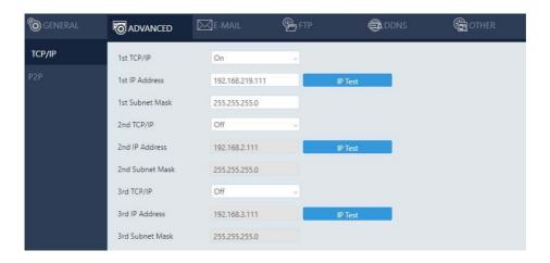
NVR supports three sets of virtual IP addresses. When **TCP/IP** is switched **On**, the NVR can access the camera or another NVR using the specific IP.
