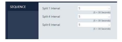
You are allowed to view videos of multiple cameras in sequence. Specify the **Sequence Interval** for the NVR to switch to the next camera or camera group for monitoring.
