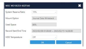
**System Reserve Ratio** allows you to allocate the percentage of HDD space that will not be occupied by recorded files. In **Mount Option**, choose the writing mode for the hard drive.
