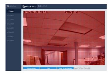
Click and drag across the grid to highlight motion detection areas. Click **Apply All Channels** to apply the areas to all camera channels.
