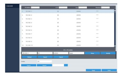
This tab allows you to cascade multiple NVRs or adjust relevant settings. For detailed instructions on how to use the NVR cascade function, visit our official website. Enter **Support > SDK**, and download the document named **DVR/NVR IR/keyboard serial commands over HTTP**. The settings listed in this tab are described in details as follows:
