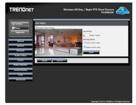
Sound detection allows the camera to pick up audio from the TV-IP862IC. When you enable sound detection, the camera listens for sounds based on the sensitivity level you created. The lower the sensitivity level the easier it is for the camera to detect sounds, thereby activating the camera to start recording.
