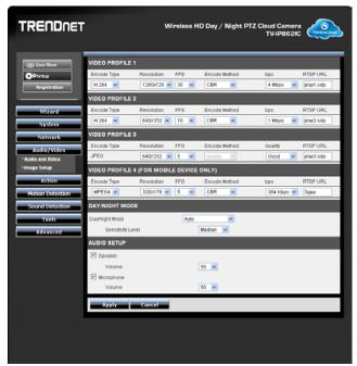
Under each profile settings there are six main functions, Encoder Type, Resolution, Frames per Second, Encode Method, bps, and RTSP URL settings.
