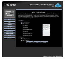
In the Static IP address field, type in the IPv4 IP Address, the Subnet Mask, Default Gateway, Primary DNS and/or Secondary DNS servers. There is also an option to include a Search Domain if you have one.
