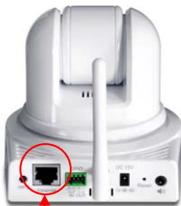
Connecting the Ethernet Cable
