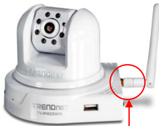
Connecting the External Antenna
