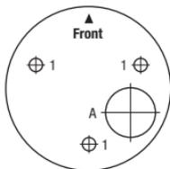
3. Drill holes for the provided screw anchors at each marked position on the template. Make sure the drill bit matches the size of the provided screw anchors.
