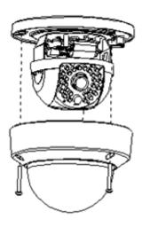
Fix the mounting base on the ceiling with the screws that come with the package. Route the cables into the ceiling or route it through the hole on the side.
