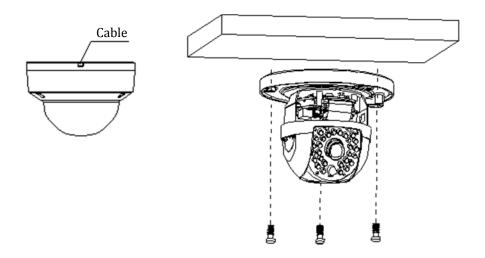
Loosen the tilt lock screws, adjust the tilting position in a range from  $15^\circ$  to  $90^\circ$ , and tighten the tilt lock screws.
