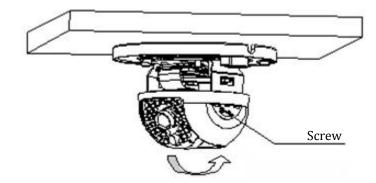
Fasten the lower dome back to the camera evenly and tightly. This step is important to block the water and dust.
