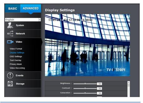
**Brightness:** Use the slider or enter a number (0-100) to adjust
