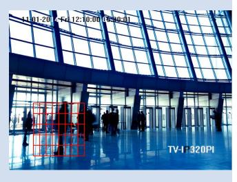
**Sensitivit** Move the slider to adjust detection sensitivity.
