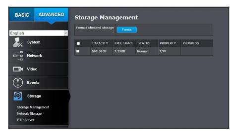
Format: Select a network storage volume and then click Format to format your network storage. This action will format the network volume (shared folder) for video recording. Placeholder files (formatting files) will be created to make sure disk allocation is appropriate and the file searching is optimized.
