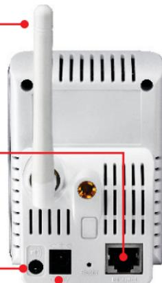
2. Connect the provided network cable from one of your Router's network ports to the **Ethernet** port on the IP Camera.
