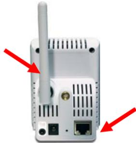
Attach the external power supply to the DC power input connector located on Camera's real Panel, and then connect it to your local power supply.
