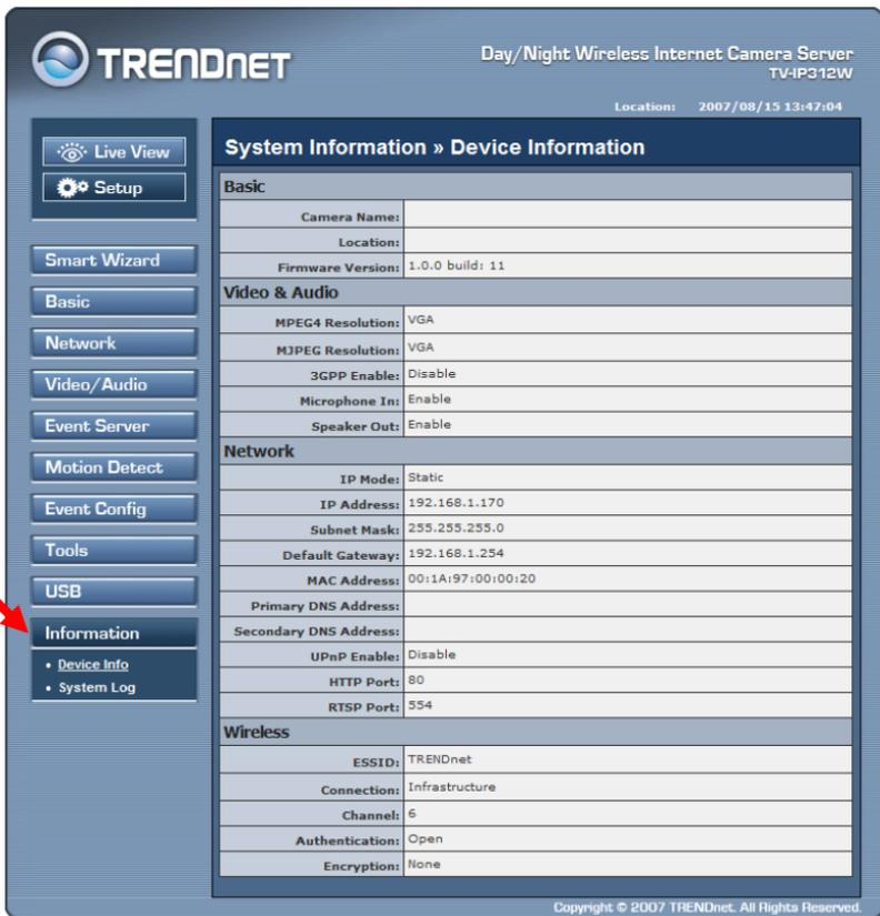
The screenshot shows the TRENDnet web interface for a Day/Night Wireless Internet Camera Server (TV-IP312W). The interface includes a navigation sidebar on the left with buttons for Live View, Setup, Smart Wizard, Basic, Network, Video/Audio, Event Server, Motion Detect, Event Config, Tools, USB, and Information. A red arrow points to the Information button. The main content area displays 'System Information » Device Information' with the following settings:
