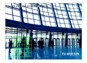
Draw Area: Click Draw Area button to start drawing. Click and drag on the area you want to set up the motion detection. You can draw up to 8 different areas. Click Stop Drawing to stop drawing motion detection areas.
