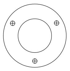
Loosen the screws with the torx screw driver which comes with the package to remove the lower dome.
