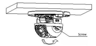
Fasten the lower dome back to the camera evenly and tightly. This step is important to block the water and dust.
