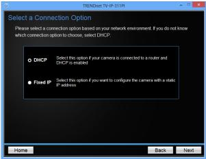
7. If you select **Fixed IP**, enter the IP address, subnet mask, default gateway, and DNS server address. Please make sure the IP address you are setting on the camera is in the same network of the computer that you are using. Click **Next**.
