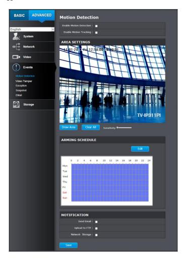
**Enable** Check this box to enable motion detection. Click **Save Motion** to save the choice.
