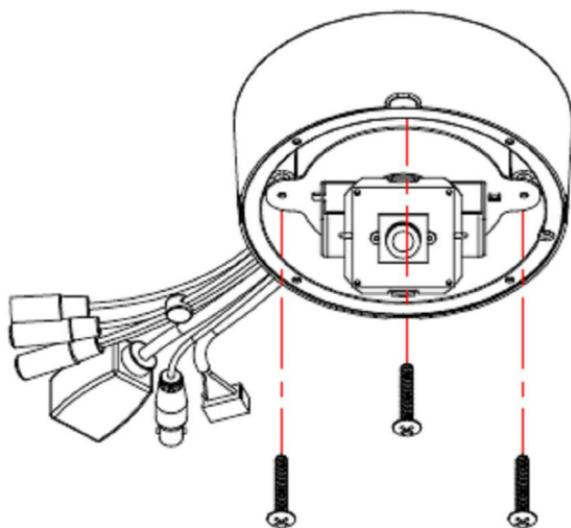
4. Make connections according to your needs (refer to the illustration of connecting cables on page 6).
