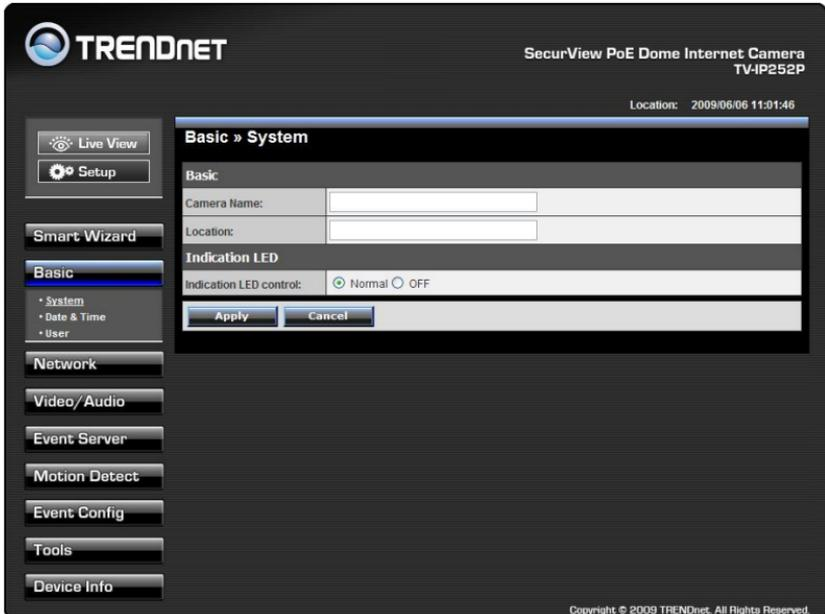
The Web Configuration contains the settings that are required for the camera in the left menu bar, including **Smart Wizard**, **Basic**, **Network**, **Video/Audio**, **Event Server**, **Motion detect**, **Event Config**, **Tools**, **USB**, and **Information**.
