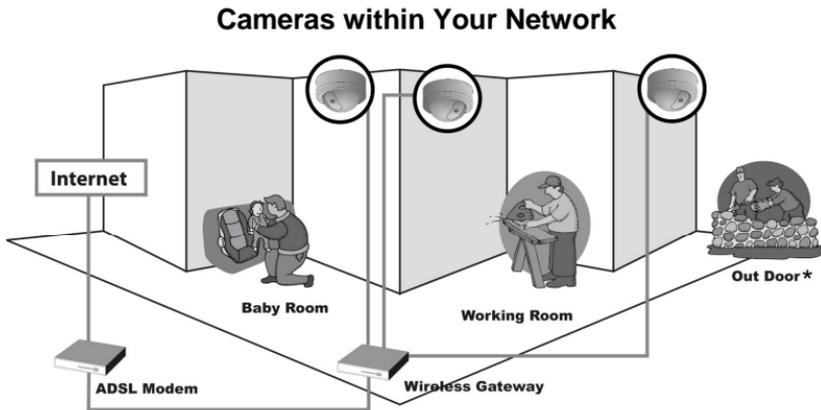
\* Please enclose with waterproof housing when using in outdoor environment. The unit itself is not weatherproof.
