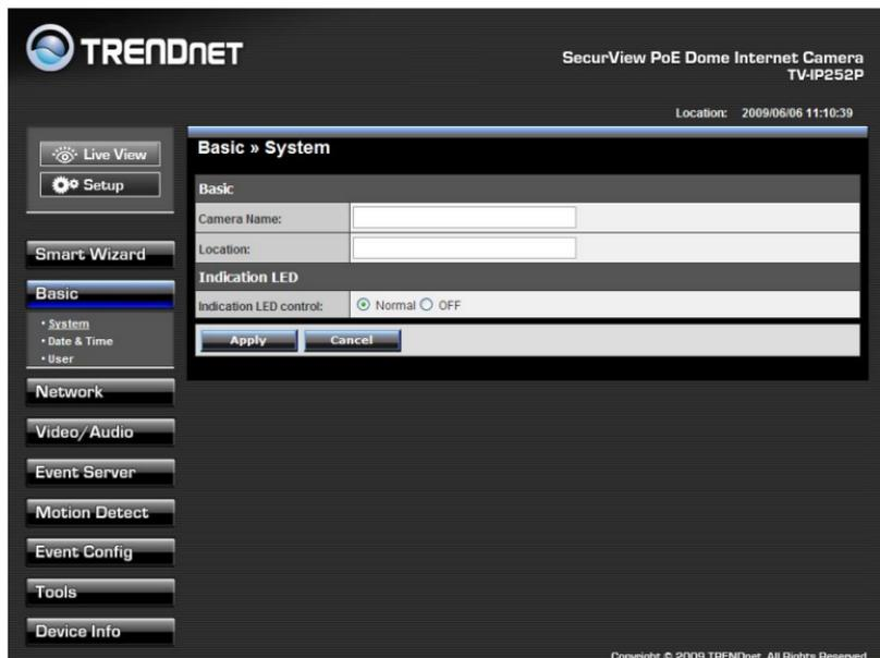
The screenshot shows the web interface for a TRENDnet SecurView PoE Dome Internet Camera (TV-IP252P). The interface includes a navigation sidebar on the left with options like Live View, Setup, Smart Wizard, Basic, Network, Video/Audio, Event Server, Motion Detect, Event Config, Tools, and Device Info. The main content area is titled "Basic » System" and contains the following configuration fields:
