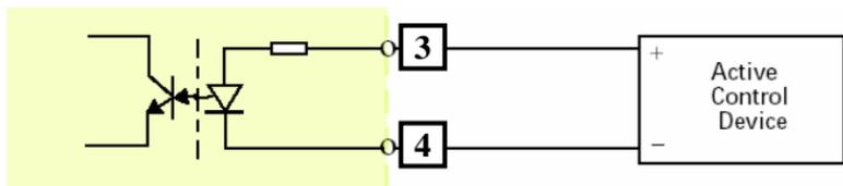
2. Output device (load) is driven by external power supply.
