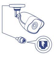
**Power over Ethernet (PoE)** PoE offers cost savings and the flexibility to install the surveillance camera up to 100m (328 ft.) from your PoE source equipment.
