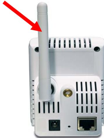
Attach the external power supply to the DC power input connector located on Camera's real Panel, and then connect it to your local power supply.
