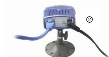
**TIP:** You can confirm power source is supplied from the LED indicators label Power on the Internet Camera is illuminated.
