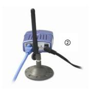
**TIP:** You can confirm power source is supplied from the LED indicators label Power on the Wireless Internet Camera is illuminated.
