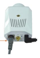
**10.** Connect the power terminal to the provided 12V DC, 0.6A power adapter.
