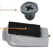
4. Connect the black bracket back inside the enclosure. Move the camera as close to the glass as possible. This example shows a TRENDnet TV-IP100W-N.
