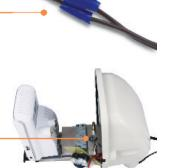
**23.** Screw the circuit board back to the metal bracket.
