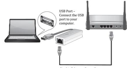
Gigabit Ethernet Port –Connect one end of the network cable to Gigabit Ethernet Port and the other end to your Gigabit Router.
