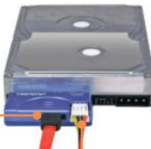
4. Connect the female Berg power connector on the provided power Y-cable to the TU-IDES.
