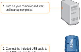
Connect the included USB cable to the USB Hub, and then to your computer's USB port.
