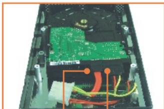
4. Connect the SATA data cable and power connector into the SATA hard drive
