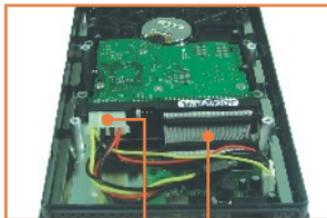
4. Connect the IDE data cable and power connector into the IDE hard drive
