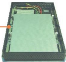
**6.** Slide the cover back on and secure it with the 4 screws.
