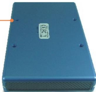
2. Remove the 4 screws to remove the metal hard drive cover.
