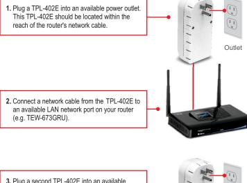
Plug a second TPL-402E into an available power outlet where your remote computer or network appliances (e.g. Game Console, IP Set box, network enabled TV, etc.) are located. 4. Connect a network cable from the second TPL-402E's network port into the network port on your remote computer or network appliance (e.g. Game Console, Blu-ray player, IP set top box, network enabled TV, etc.).
