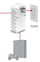
Verify that the PWR (Power), PL (Powerline) and ETH (Ethernet Link/Act) LEDs are on for both TPL-402E adapters.
