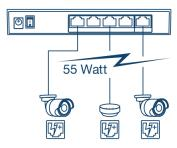
2.5G Ports Equipped with 2.5GBASE-T RJ-45 ports that provide higher gigabit speeds capable of up to 2.5Gbps over existing Cat5e or better cabling. Wall Mountable The 2.5G PoE+ switches feature a metal housing with a convenient wall mountable design for greater installation flexibility. **PoE+** A 55W total PoE power budget on this PoE+ switch supplies up to four PoE+ devices with up to 30W per port.
