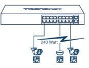
Hardware Design With a sturdy metal housing and rackmount brackets included, this switch is well-suited for 19" 1U rack installations. **PoE Power** A 240W total PoE power budget supports 16 PoE+ devices with up to 30W per port.
