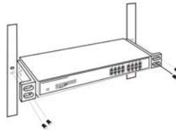
Figure 2. Mount the Switch in the rack
