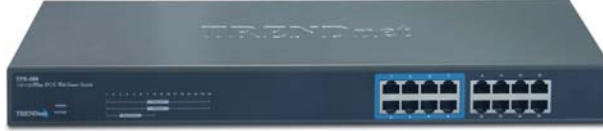
Figure 3. Front panel of 16-port Gigabit Ethernet Switch with 8-port PoE
