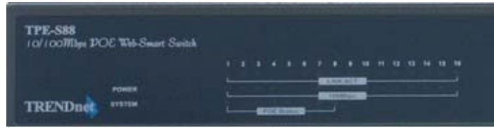
Figure 5. LED indicators of the Switch
