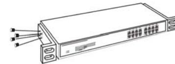
Figure 1. Combine the Switch with the provided screws
