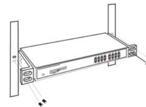
Figure 2. Mount the Switch in the rack
