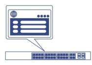
Web Smart Management Provides an easy-to-use web-based management interface to reduce switch configuration complexity and offers a combination of SMB management features for easy deployment.
