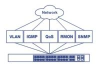
Integration Flexibility Managed features include access control lists, VLAN, IGMP snooping, QoS, RMON, SNMP trap, and syslog for monitoring and flexible network integration.
