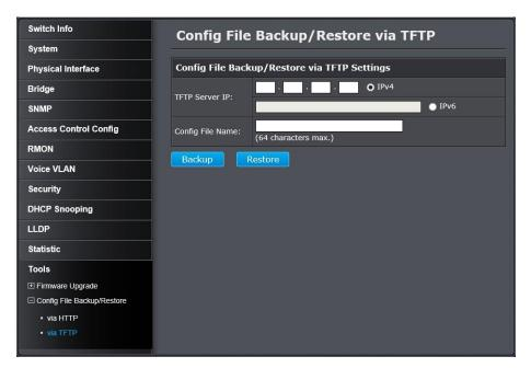
Make sure your TFTP server is running and note the IP address of your server and firmware file name. The TFTP server should be in the same IP subnet as the switch.
