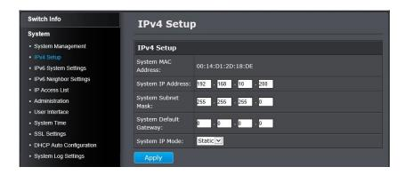
6. Configure the switch IP address settings to be within your network subnet, then click **Apply**.
