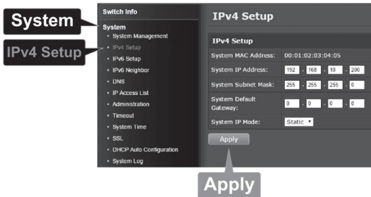
The screenshot shows the 'IPv4 Setup' configuration page. On the left, a 'System' menu is open, and 'IPv4 Setup' is selected. The main area shows the following configuration:
