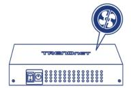
**4-Port PoE** The 4-port gigabit PoE+ injector supplies up to 30W of power to four PoE or PoE+ devices.
