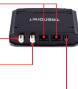
5. Verify that PWR, LAN1 or LAN2 and HPNA LEDs are lift.
