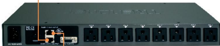
2. Connect the opposite end of the RJ-45 Ethernet cable to the **Daisy Chain Input** port on the second TK-RP08 (slave).
