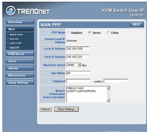
PPP Connection over direct serial cable with TK-IP101 as PPP Server
