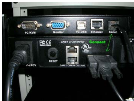
A real connection case of TK-RP08 and TK-IP101 Trendnet KVM back panel
