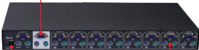
3. Connect the included AC Power Adapter to the KVM switch and then to a power outlet.
