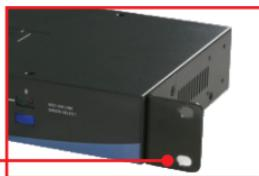
12. Carefully position the switch onto the rack. Align the bracket to the screw holes on the rack, then use the screws provided with the equipment rack to mount the switch.
