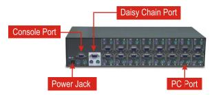
**Console Port -** Connect to your shared keyboard, monitor, and mouse. **PC Port -** Connect to your computer's keyboard, video and mouse cable. **Daisy Chain Port -** For stacking to another TK-802R or TK-1602R KVM switch (console port).
