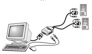
**DO NOT** connect the KVM cable to a computer that is still power-on. The computer will have difficulty recognizing the shared keyboard and mouse.
