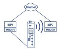
**Dual-WAN** Connect up to two separate WAN internet connections (Ethernet & WiFi) to efficiently load-balance traffic, or configure for redundancy using the WAN fail-over mode.
